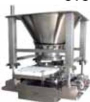
The **TIP SYSTEM** is a revolutionary connection system for the obtainment of a high level of containment. OEL - (Operator Exposure Level)  $1\mu/m^3$ . It is completely automatic and ensures a perfect seal between two machines. Suitable for C.I.P. (cleaning in place).
